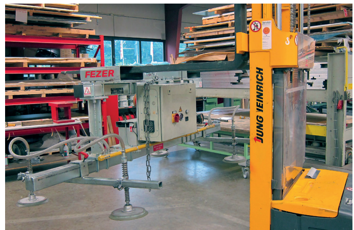
VacuBoyForker VB-250KG for the transfer of steel sheets
